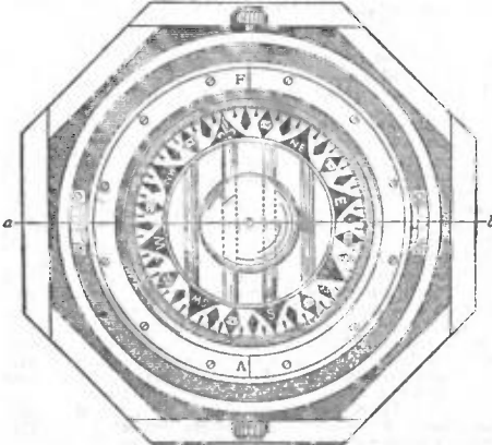
FIG. 4.—Abbe's Marine Nephoscope. Horizontal Projection of Compass.
